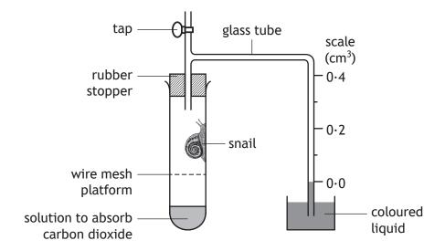
The experiment was carried out at 10 °C, 15 °C, 20 °C and 25 °C. At each temperature, the tap was left open for 15 minutes then closed and readings were taken from the scale every 2 minutes.
