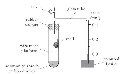
The apparatus was kept at  $10\,^{\circ}\text{C}$  with the tap open for 15 minutes. To start the experiment, the tap was closed and the reading on the scale recorded.
