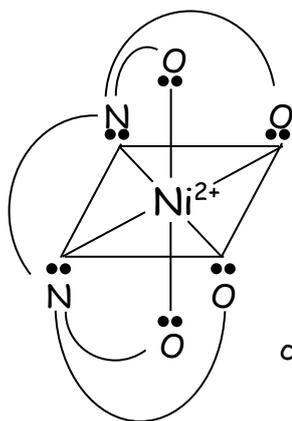
Hexadentate EDTA complexing with  $\text{Ni}^{2+}$  ion
