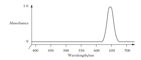
The absorption spectrum of a solution of sodium tetrachlorocobaltate(II) is shown above.
