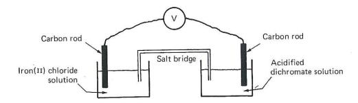
In acid solution, dichromate ions  $(Cr_2O_7^{2-}(aq))$  are reduced to  $Cr^{3+}(aq)$  ions.
