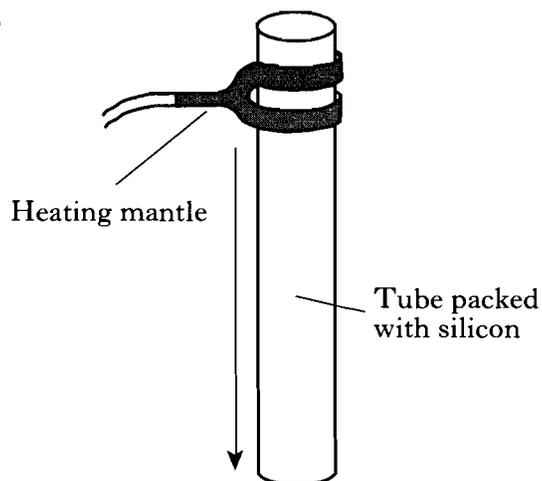
Ultra pure silicon for silicon chips is obtained by zone refining. This process involves passing a heating coil down a tube packed with silicon which is already fairly pure.
