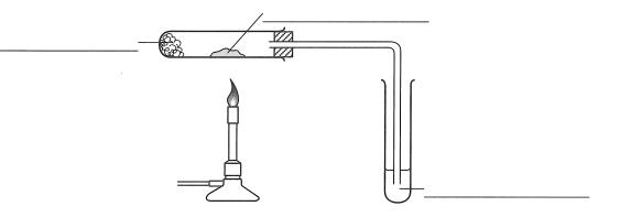
(a) Label the diagram of the apparatus used to crack liquid paraffin.
