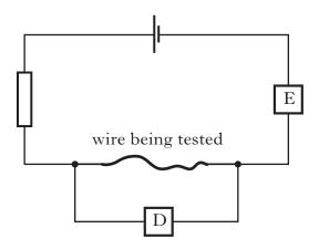
(a) At which position in the circuit should an ammeter be placed, D or E?
