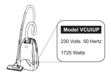
(a) Calculate the current in the vacuum cleaner when it is switched on.
