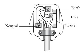
Complete the table below to identify the colours of the insulation on the wires inside the plug.
