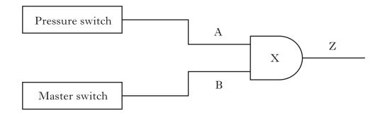
Pressure switch when closed gives logic 1 Pressure switch when open gives logic 0
