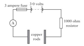
A student holds a copper rod in each hand and notes the reading on the ammeter.
