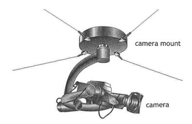
The camera mount is suspended from four cables. The length of the cables can be changed using a motor attached to each cable. This allows the height and position of the camera over the pitch to be changed.
