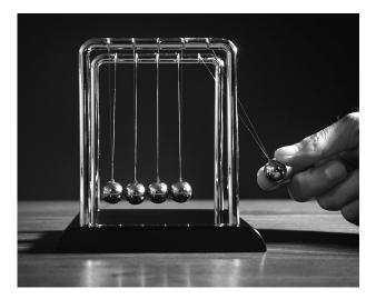
The ball at the end is raised and then released, striking the closest of the four stationary balls.
