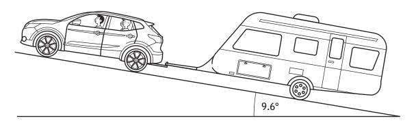
(a) (i) Determine the component of the total weight of the car, passengers, and caravan acting down the slope.
