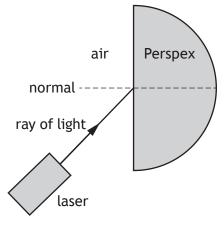
(a) The student measures a number of different angles of incidence  $\theta_i$  and the corresponding angles of refraction  $\theta_r$ .
