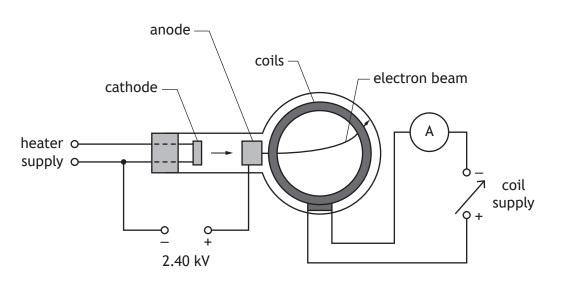
(a) The heater supply is used to heat the cathode, which causes electrons to be released from its surface.
