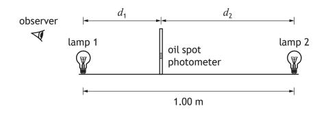
The oil spot photometer is a piece of card with an oil spot on it, which is used to compare the brightness of two light sources on either side of the photometer. When the relative brightness of the light on either side of the photometer is equal, no spot is observed.
