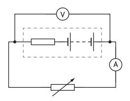
The resistance of the variable resistor is changed and the corresponding readings on the ammeter and voltmeter are used to produce the graph shown.
