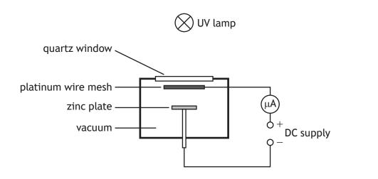
When the lamp is switched on, ultraviolet (UV) radiation passes through the quartz window and wire mesh, and is incident on the zinc plate.
