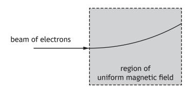
Determine the direction of the uniform magnetic field.
