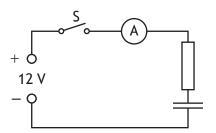
The capacitor is initially uncharged.
