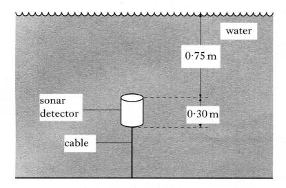
The detector has a mass of  $100 \,\mathrm{kg}$ . Each end of the detector has an area of  $0.40 \,\mathrm{m}^2$ . Atmospheric pressure is  $101 \,000 \,\mathrm{Pa}$ .
