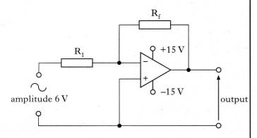
Which values for resistors  $R_1$  and  $R_f$  will produce an approximate square wave output?
