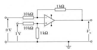
What is the value of the output voltage  $V_0$ ?
