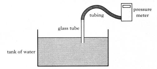
The pressure meter is set to zero before the glass tube is lowered into the water.
