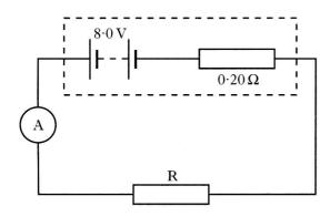
The reading on the ammeter is  $4.0 \,\mathrm{A}$ .
