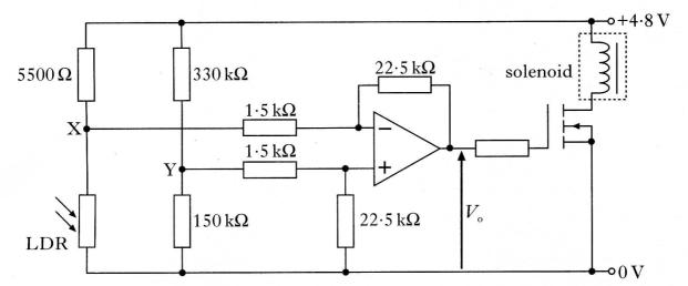
The potential at Y is  $1.50\,\mathrm{V}$ . When the washing machine is filling with water, the narrow beam of light illuminates the LDR, the bridge is unbalanced and the potential at X is  $1.28\,\mathrm{V}$ .
