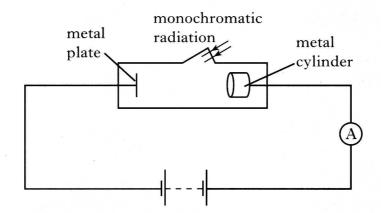
There is a constant potential difference between the metal plate and the metal cylinder.
