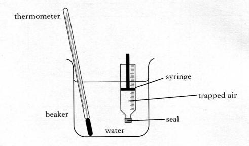
The volume of the trapped air is read from the scale on the syringe.
