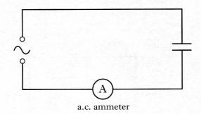
The alternating supply has a constant peak voltage but its frequency can be varied.
