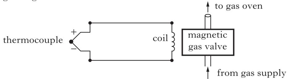
When the current in the coil is less than  $2.5 \text{ A}$ , the gas valve is closed.
