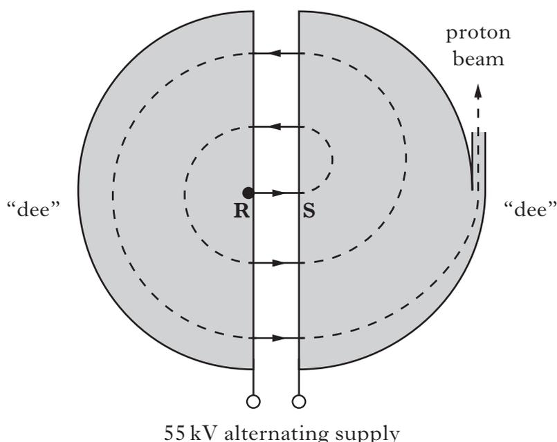
Protons are released from rest at **R** and are accelerated across the gap between the “dees” by a voltage of 55 kV.
