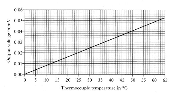
(i) What is the voltage produced by the thermocouple at 37 °C?
