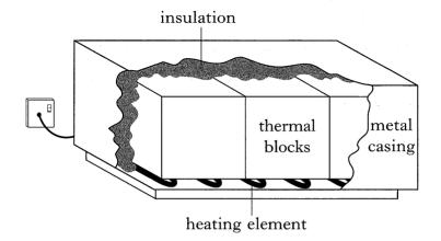
The heating element heats the thermal blocks during the night.
